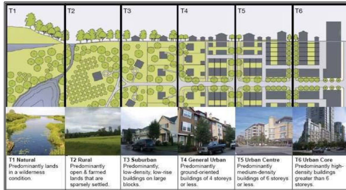
New Urbanism Typical Transect Progression Diagram with photo examples
