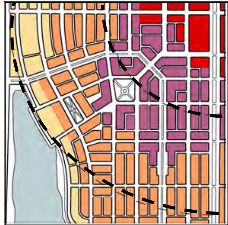
Quarter-section of the Community Center TOD Station Area with radii at 1/4-mile and 1/2-mile, showing general concept of street grid, form, and general land use concept showing:
