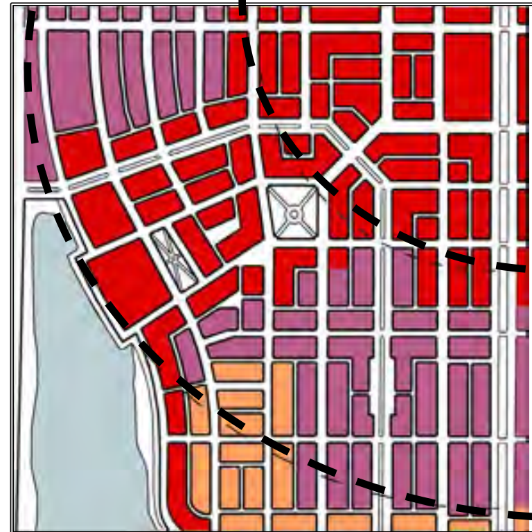
Quarter-section of the Regional Center TOD Station Area with radii at 1/4-mile and 1/2-mile, showing general concept of street grid, form, and general land use concept showing:
